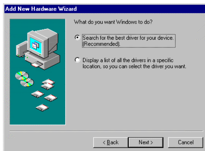
Figure 7: Choosing the way of driver installation
